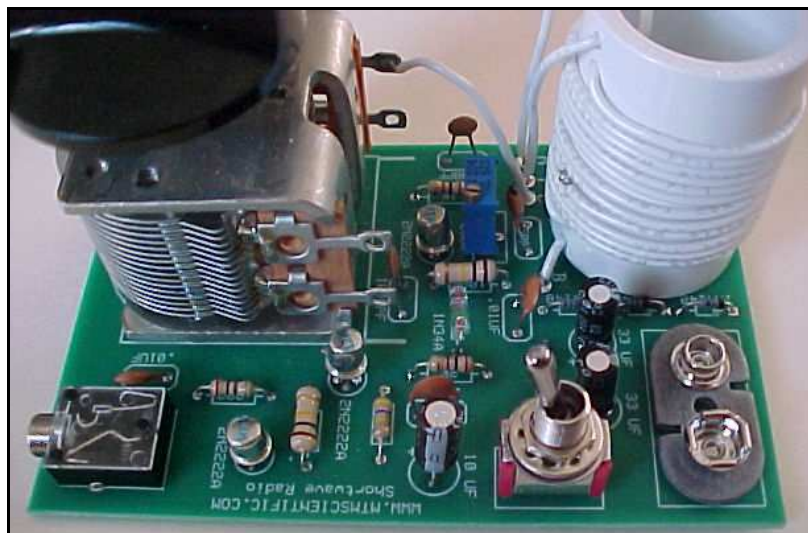
Fig 12: Detailed view of assembled kit from another angle. The wire from the air variable capacitor to the board location 'T' is visible
