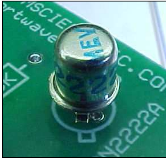
Fig 3: Insert the transistors with the tab aligned with the board art.
