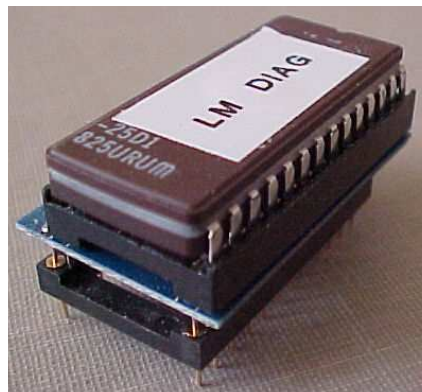
Figure 14. The diagnostic program can be burned on a 27XXX series chip and installed in socket U33 (BIOS Socket) by using an adapter.
