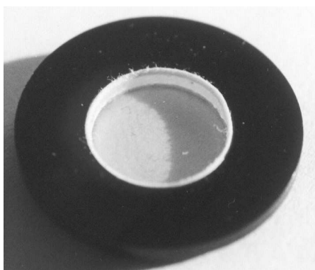
Figure 2. Masking tape around the edges of a small lens makes for a perfect fit.
